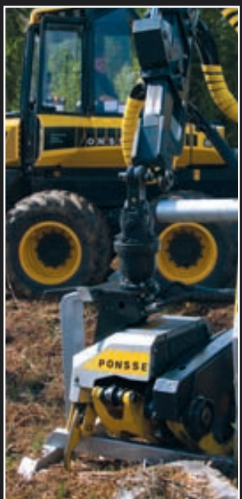
The boom's quick mounting bracket guides the harvester head easily into place and locks the mounting.
