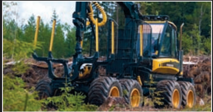
Modification from a forwarder to a harvester or visa versa takes only a couple of minutes. If necessary, the log gate, bunks and rear frame extension are removed from the forwarder for harvesting.
