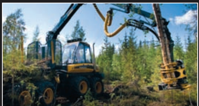
Trees can be piled or lifted directly to the loading space for the Dual machine.
