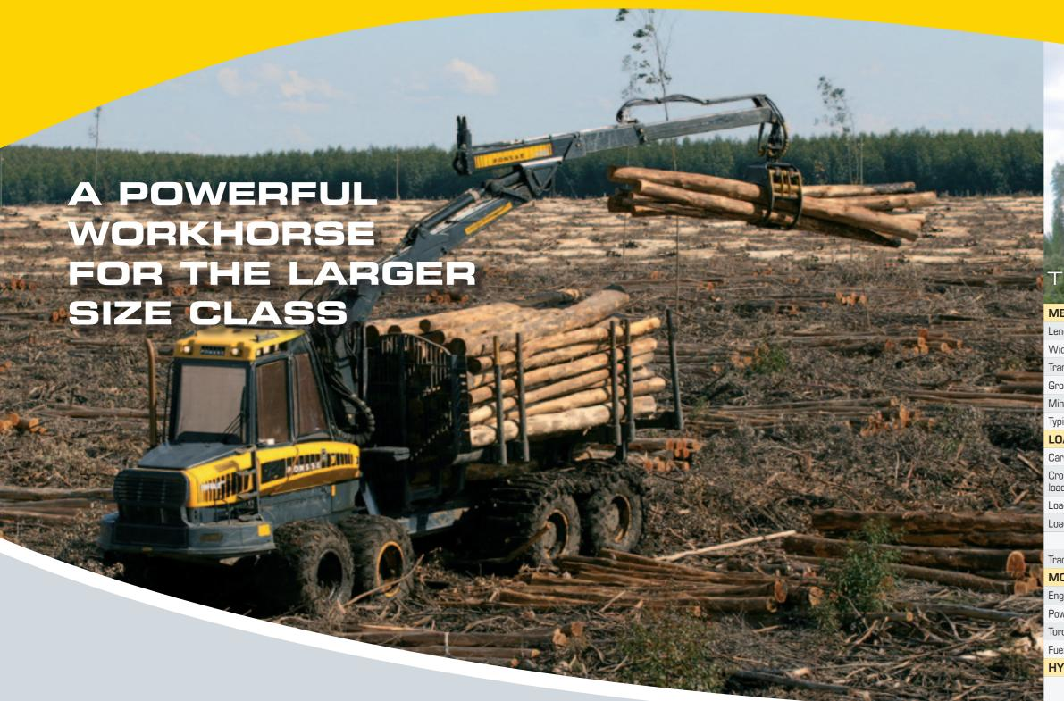
PONSSE BuffaloKing can carry nearly its own weight in wood and provides its operator with a luxurious cab, a powerful PONSSE K100+ crane, a large carrying capacity, a powerful Mercedes-Benz engine and a strong frame — everything needed for harvesting timber on the most demanding scale in the larger size class!
